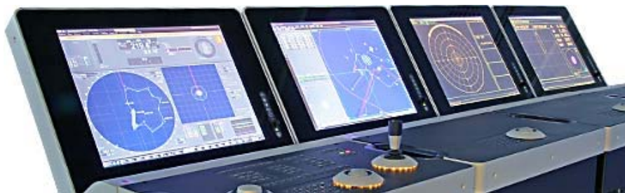
Figure 28: Dynamic Positioning system
