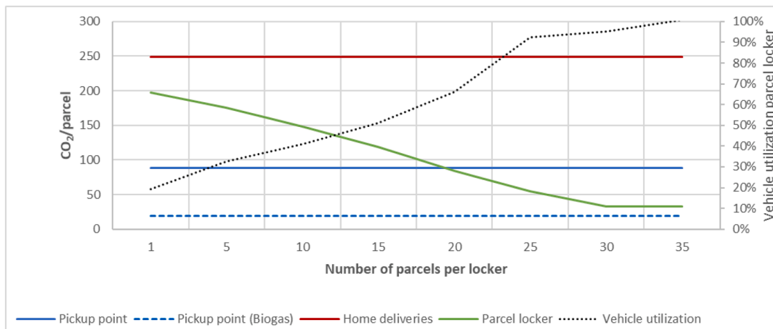
Fig. 4.3. Analysis of how changes in the delivered number of parcels per locker affect CO 2 emissions per parcel, compared to the other delivery solutions.
