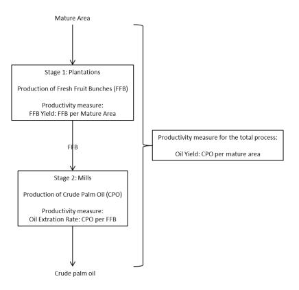
Figure 4: Production process of Crude Palm oil
