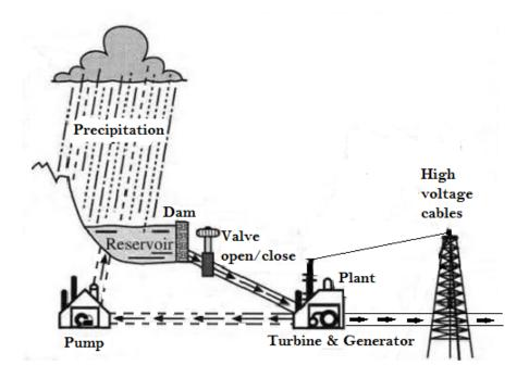
Figure 5: Generation of hydro-electricity by a high-head power plant
