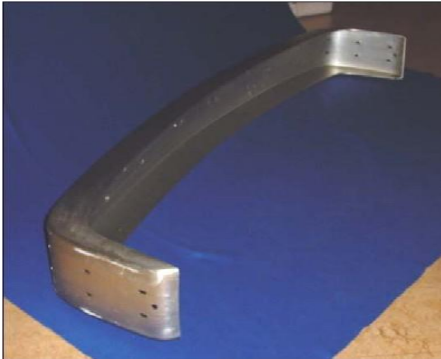
Figure 3-5 The bumper for the Volvo 140 series after the development of the "strong" alloy (image from RA's archive)
