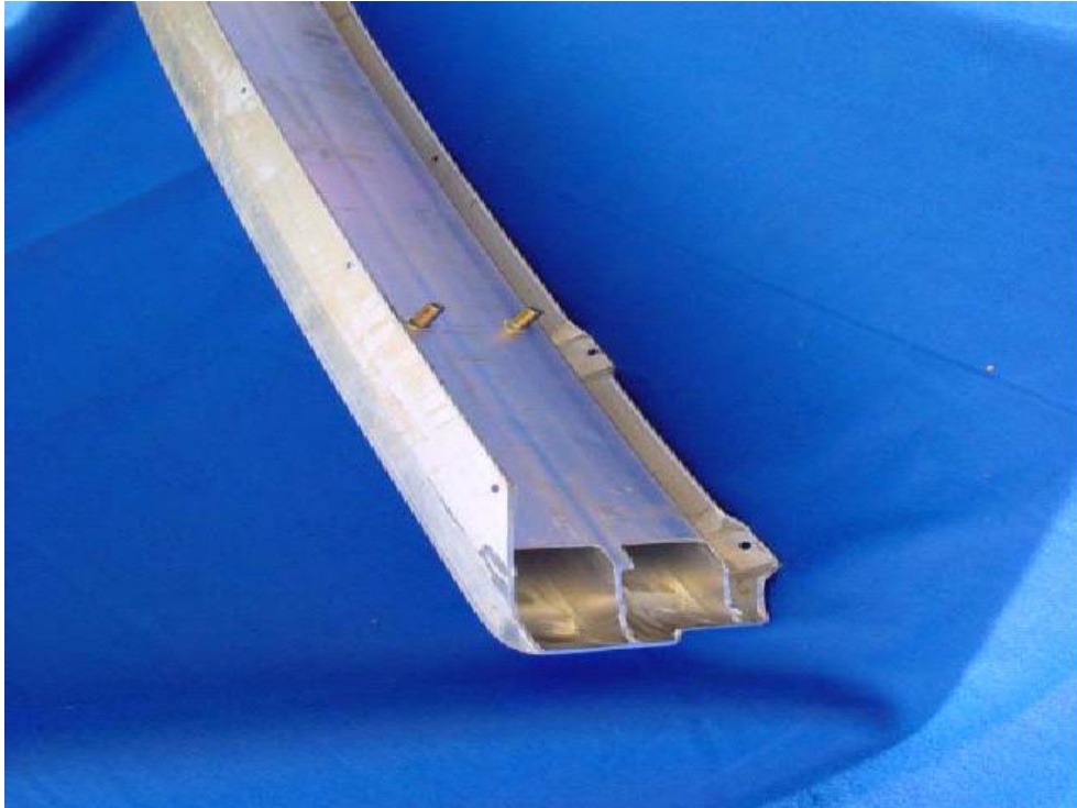
Figure 3-10 The first hollow bumper beam made for the Volvo 740 (image from Bjørn-Anders Hilland)
