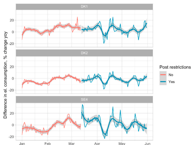
Fig. 6. Percentage change in electricity consumption, year-over-year with a Loess smoothed curve overlapped.
