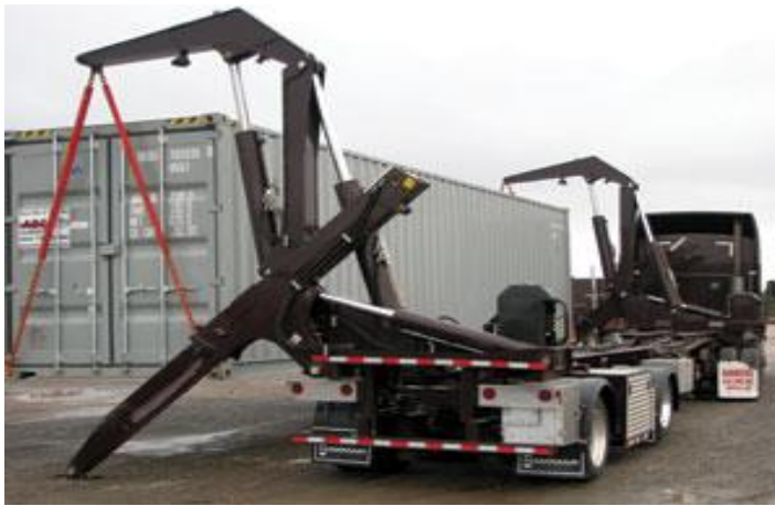
Figure 7.6 - Container placed at ground level
