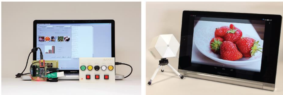
Figure 2. Left: Digital Taste Interface: A method for simulating the sense of taste by actuating the human tongue through electrical and thermal stimulation (Ranasinghe, Karunanayaka, Cheok, Fernando, Nii, & Gopalakrishnakone, 2011). Right: AromaShooter, a smell-delivery device, contains six scent cartridges and connects to a computer via USB. (Developed by Aromajoin)
