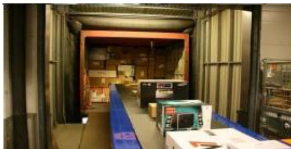
Picture 27: Conveyer belt directly into the truck
