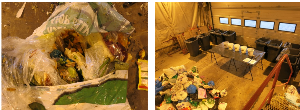
Figure 5-6: Example of a residual waste bag cut open during the residual waste analysis (left). All of the residual waste bags were sorted into their respective waste fractions (right).
