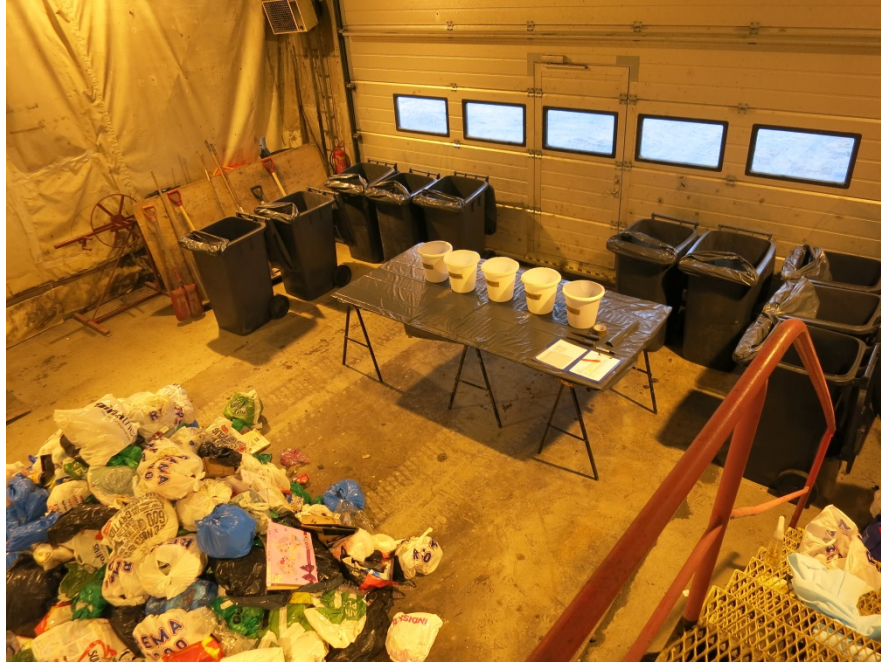
Picture 1: Pick-analysis set-up with sorting table, buckets and 240l containers lined up around.
